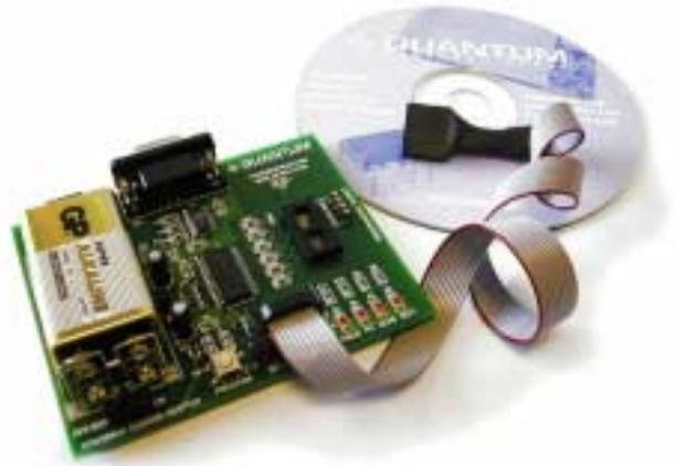
For production use, the target PCB can have a similar connector which allows the QTM300CA to upload settings on a mass basis. The cloning process takes under 1 second to complete.
